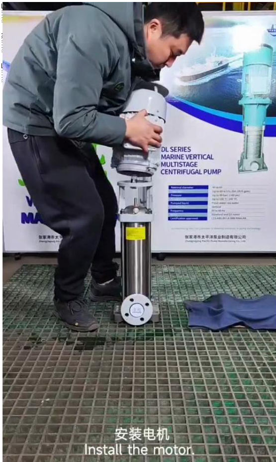
安装电机座 Install the motor stool.
